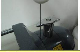
Test for protection against access to hazardous parts
